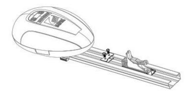
Using screw M6.3\*20 fix the track with motor head through the U shaped buckle for added strength to ensure the mechanism doesn't move.
